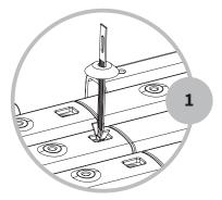
Line up arrow with insertion slot and push the QuickZip arrow through both panels.
