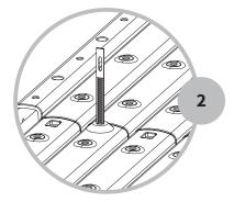
Pull up on the QuickZip and push down the tightening cap tight – ensuring the zip tie teeth catch. Trim off any extra tie length.
